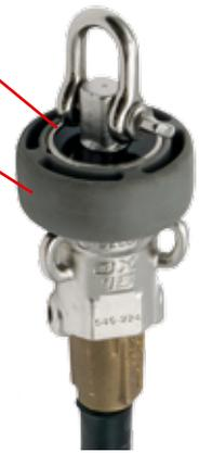
Impact resistant composite cover around the line driver keeps the line in order and prevents damage to the boat when handling the system on the foredeck.
