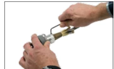
Install the drum/halyard swivel and tighten the locking screw.
